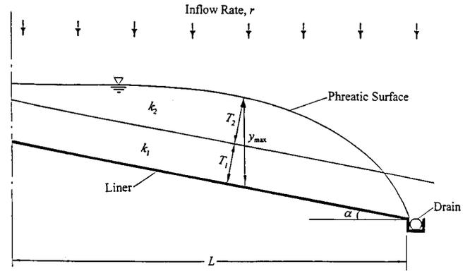
Fig. 16. Phreatic surface in two-layered drainage media, typical of leachate collection and cover soil drainage situations
