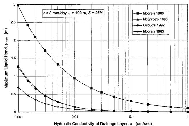
**Fig. 10.** Relationship between maximum liquid head and hydraulic conductivity of drainage layer for landfill cover from different calculation methods
