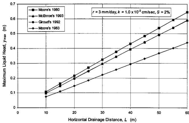
**Fig. 3.** Relationship between maximum liquid head and horizontal drainage distance for landfill cell from different calculation methods
