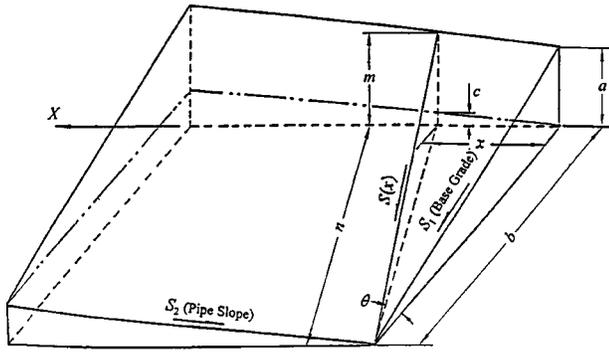
Fig. 11. Landfill cell floor grade
