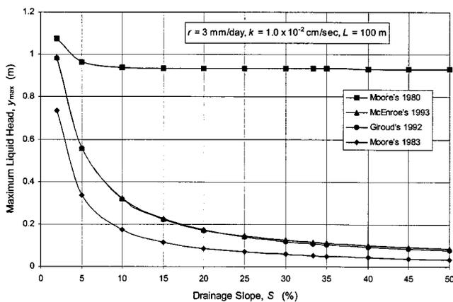
**Fig. 8.** Relationship between maximum liquid head and drainage slope for landfill cover from different calculation methods
