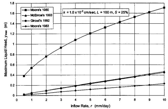
**Fig. 9.** Relationship between maximum liquid head and inflow rate for landfill cover from different calculation methods
