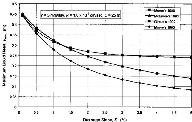
**Fig. 4.** Relationship between maximum liquid head and drainage slope for landfill cell from different calculation methods
