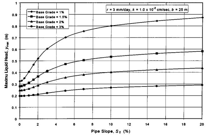
**Fig. 13.** Effect of pipe slope on maximum liquid head with various landfill base grades
