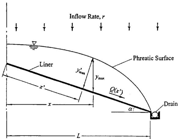
Fig. 1. Phreatic surface in landfill drainage layer
