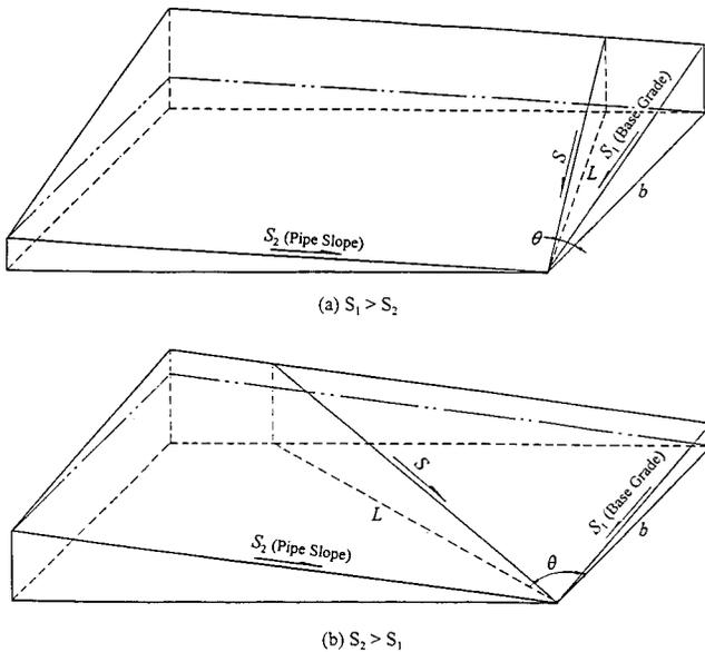
**Fig. 12.** Actual leachate flow grade and horizontal drainage distance for different combinations of base grade and pipe slope: (a)  $S_1 > S_2$  and (b)  $S_1 < S_2$
