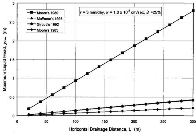
**Fig. 7.** Relationship between maximum liquid head and horizontal drainage distance for landfill cover from different calculation methods
