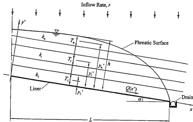
Fig. 15. Phreatic surface in multilayered drainage media
