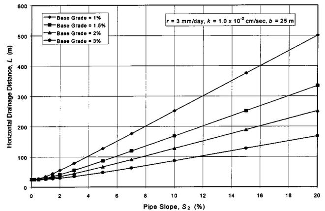
**Fig. 14.** Effect of pipe slope on horizontal drainage distance with various landfill base grades
