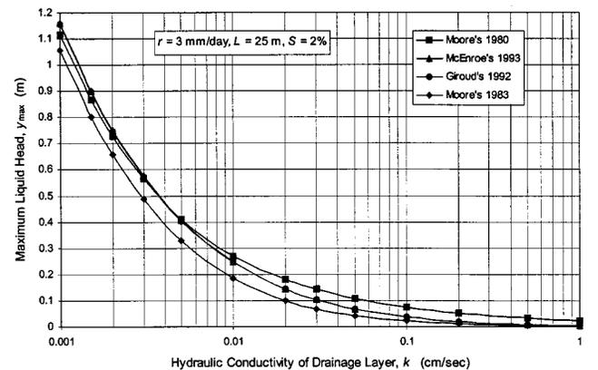
**Fig. 6.** Relationship between maximum liquid head and hydraulic conductivity of drainage layer for landfill cell from different calculation methods
