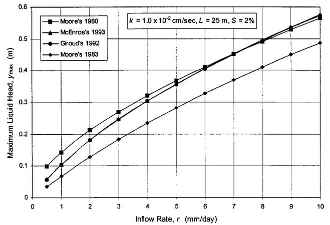
**Fig. 5.** Relationship between maximum liquid head and inflow rate for landfill cell from different calculation methods
